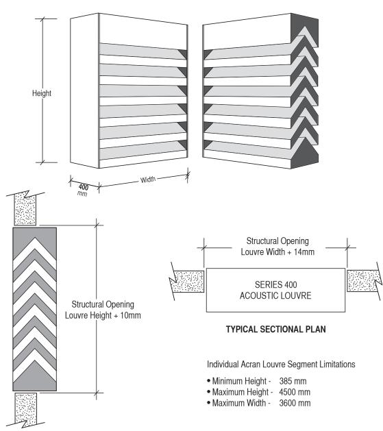
TYPICAL SECTIONAL ELEVATION
